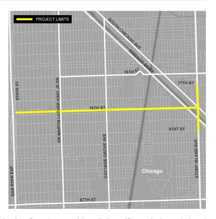
pavement markings and signage, bus stop optimization (locations and lengths), traffic analysis and signal timing improvements for transit operations, pedestrian countdown timers, and leading pedestrian intervals.
